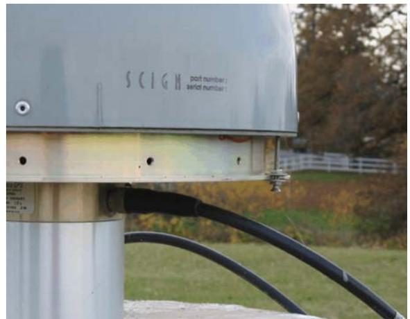
**Figure 3.** Raised dome for PGC5. The two panels show the details of mounting the SCIGN dome raised by 3.6cm
