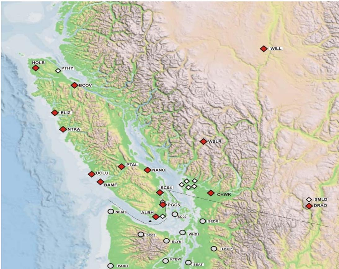
**Figure 4.** Location of continuous GPS stations included in routine daily data analysis. Shaded (red) diamonds, open diamonds, and open circles show sites from the WCDA, BCACS, and PANGA networks respectively. The GPS site at Penticton (DRAO) is used as a fixed reference site in the GPS analysis.
