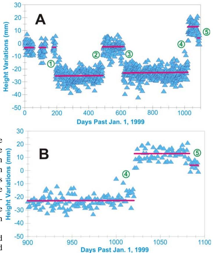
**Figure 5.** Apparent changes in height at PGC5 wrt DRAO at times of dome changes. Numbers refer to dome changes listed in Table 2. Panel B shows the last two changes (4 and 5) in greater detail. Generally, the presence of a dome delays GPS signals and thereby reduces height estimates since orbits are held fixed.
