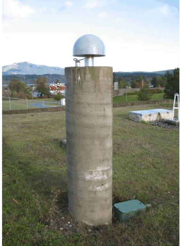
**Figure 2.** PGC5 antenna with a SCIGN short dome. The dome is held in place using the base ring-mount attached to the outer edge of the antenna groundplane. View is looking north from the PGC4 monument.
