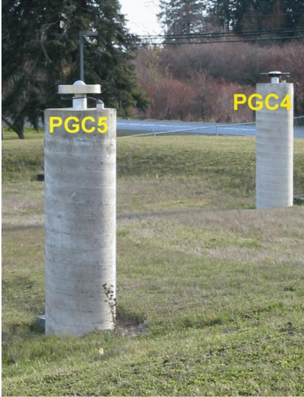
**Figure 1.** Forced-centre concrete pillar monuments for continuous GPS sites PGC4 and PGC5. PGC4, operated by the Base Mapping and Geomatic Services Branch of British Columbia, uses a Trimble micro-strip antenna with an extended ground-plane. PGC5, operated by the Geological Survey of Canada, uses a Dorne-Margolin choking antenna. Each antenna is mounted on a 10 cm stainless-steel collar that permits antenna rotation. The monuments are about 14 m apart.
