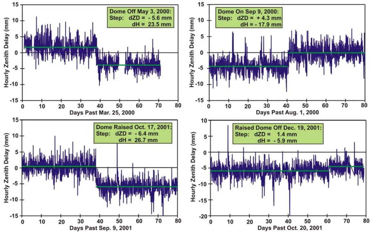
**Figure 6.** Differential (PGC5-PGC4) Zenith Delay (ZD) estimates. Changes in the hourly ZD estimates at PGC4 are subtracted from those at PGC5. Offsets are estimated by differencing 20 to 40 point averages before and after dome changes. The four panels correspond to actions 2 through 5 listed in Table 2.
