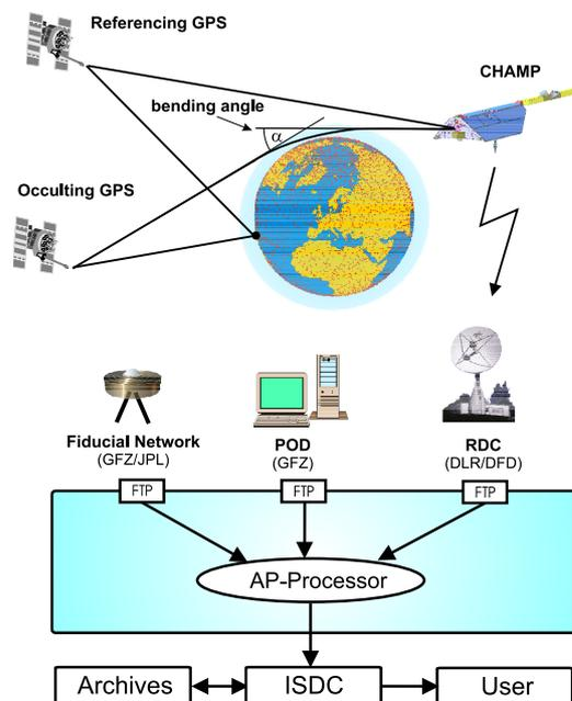
Fig. 1: Infrastructure for Atmospheric Profiling with CHAMP
