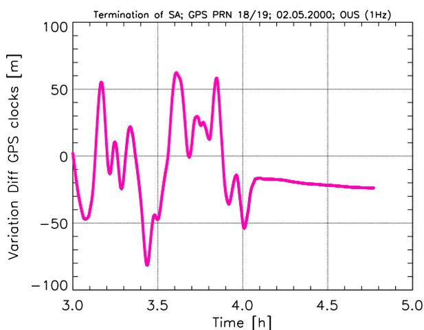
Fig. 4 Variation of GPS clocks during termination of SA (02/05/00)
