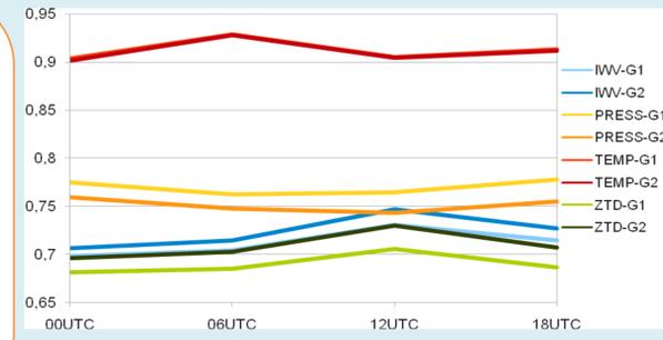
Figure 4. Correlation of observation and model results for integrated water vapour (IWV), surface pressure (PRESS), surface temperature (TEMP) and zenith total delay (ZTD).
