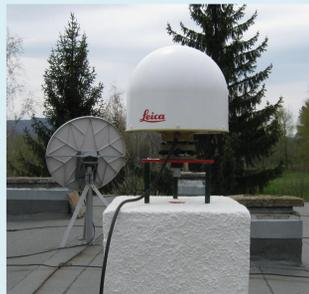
Figure 2. GNSS antenna at Sofia station.
