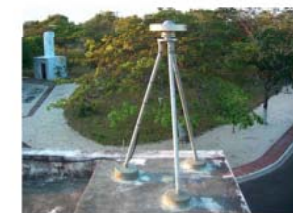
Fig. 4 This view of the BRF1 antenna and mount, taken during its installation in September 2005, is towards north. The steel tripod stands about 1.5 m tall up to the bottom connection plate.
