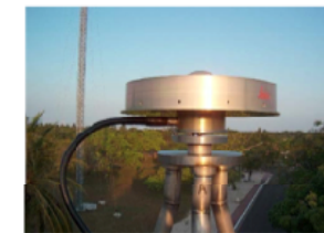
Fig. 5 Photograph showing a close-up view of the tripod top, SCIGN leveling mount, and Leica LEIAT504 chocking antenna.
